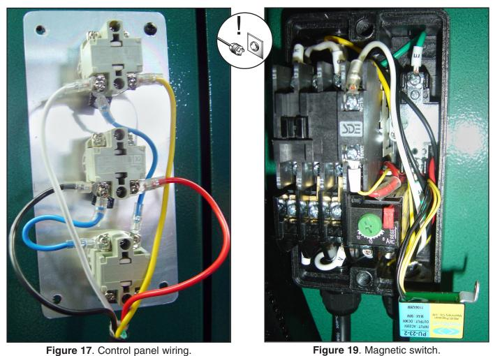
Figure 17. Control panel wiring.
